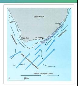
Horizontal current shear can lead to convergence of ray paths.
