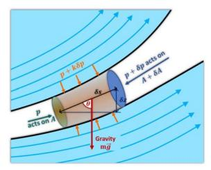
The force on an element in the direction of the flow is
