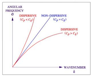
Phase velocity,  $c_p=\frac{\sigma}{k}$  ; Group velocity,  $c_g=\frac{\partial\sigma}{\partial k}$
