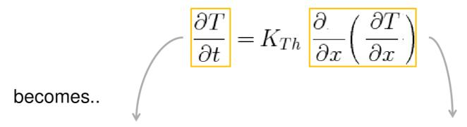
$$\frac{T_i^{n+1} - T_i^n}{\Delta t} = K_{Th} \frac{T_{i+1}^n - 2T_i^n + T_{i-1}^n}{\Delta x^2}$$
