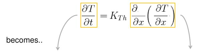
$$\frac{T_i^{n+1} - T_i^n}{\Delta t} = K_{Tv} \frac{T_{i+1}^n - 2T_i^n + T_{i-1}^n}{\Delta x^2}$$
