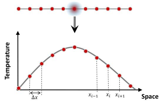
$$\frac{\partial T}{\partial x} = \frac{T_{i+1/2}^n - T_{i-1/2}^n}{\Delta t}$$
